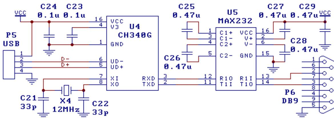
**7.3 USB to RS232 Serial Port, Simplified Version (Figure Below)**
