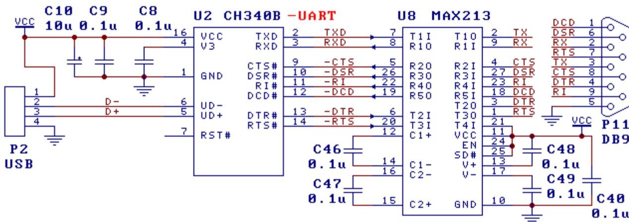
**7.2 USB to RS232 Serial Port (Figure Below)**
