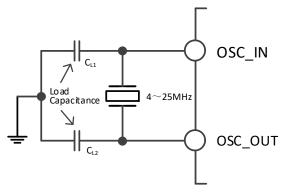
Note: The load capacitor needs to be as close to the oscillator pin as possible and the capacitance value should be selected according to the crystal manufacturer's parameters.
