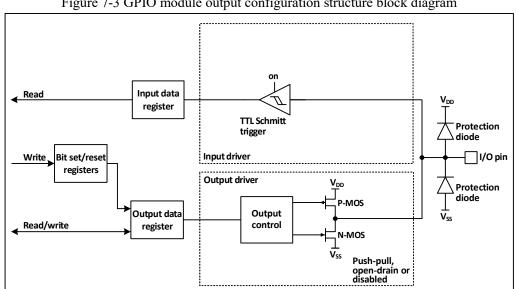
Figure 7-3 GPIO module output configuration structure block diagram
