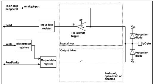
When the analog input is enabled, the output buffer is disconnected, the input of the Schmitt trigger in the input driver is disabled to prevent the generation of consumption on the IO port, the pull-up and pull-down resistors are disabled, and the read input data register will always be 0.
