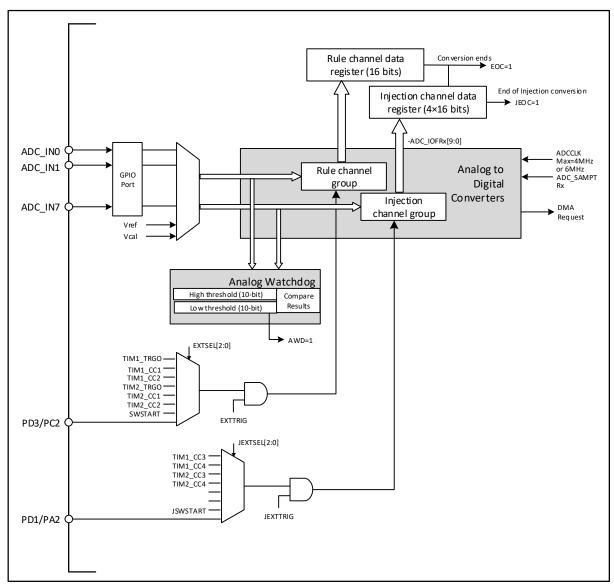
Figure 9-1 ADC module block diagram
