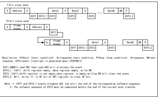
Figure 13-6 Slave transmitter transmission sequence diagram
