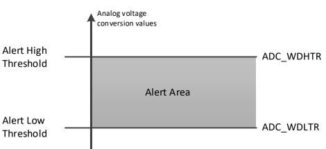
Figure 9-4 Analog watchdog threshold area
