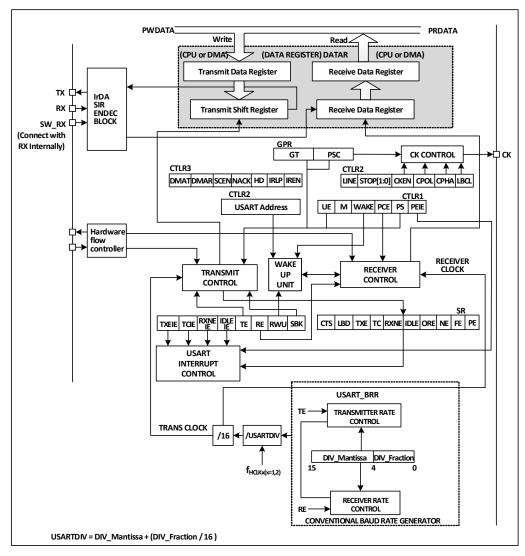
When TE (transmit enable bit) is set, the data in the transmit shift register is output on the TX pin and the clock
