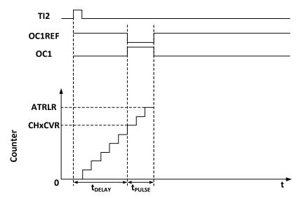
As shown in Figure 11-4, a positive pulse of length Tpulse needs to be generated on OC1 after a delay Tdelay at the beginning of a rising edge detected on the TI2 input pin.
