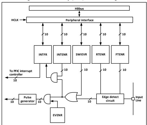
Figure 6-1 External interrupt (EXTI) interface block diagram
