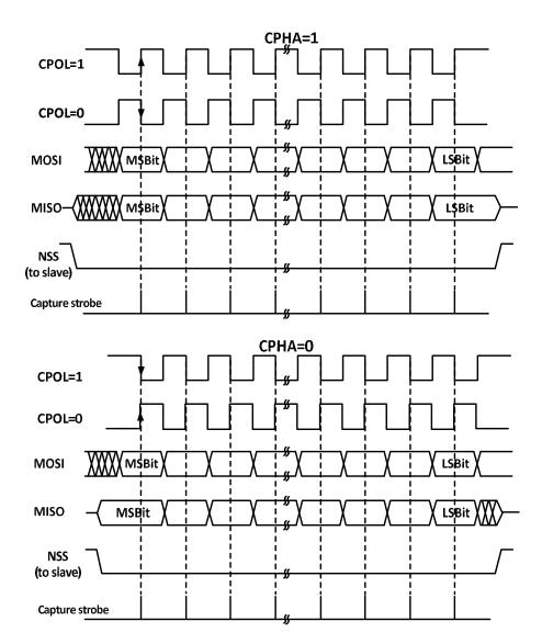
The host and device need to be set to the same SPI mode, and the SPE bit needs to be cleared before configuring the SPI mode. the DEF bit determines whether the individual data length of the SP is 8 bits or 16 bits. LSBFIRST controls whether a single data word is preceded by the high bit or the low bit.
