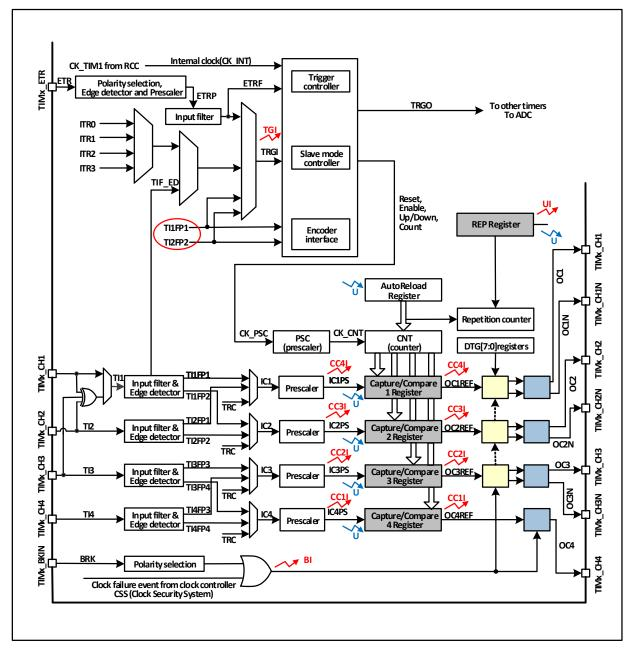
Figure 10-1 Block diagram of advanced-control timer structure
