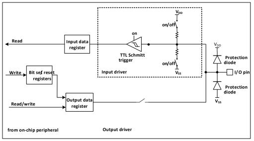
When the IO port is configured in input mode, the output driver is disconnected, the input pull-up and pulldown are selectable, and no multiplexed functions or analog inputs are connected. The data on each IO port is sampled into the input data register at each HB clock, and the level status of the corresponding pin is obtained by reading the corresponding bit of the input data register.
