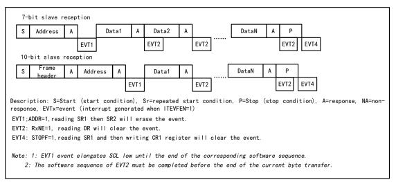
The master device will generate a stop condition after the last data byte is transferred. When the I2C module detects a stop event, it will set the STOPF bit, and if the ITEVFEN bit is set, it will also generate an interrupt. The user needs to read the status register (R16\_I2Cx\_STAR1) and then write the control register (e.g. reset control word SWRST) to clear it. (See EVT4 in the figure above).
