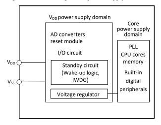
Figure 2-1 Block diagram of power supply structure
