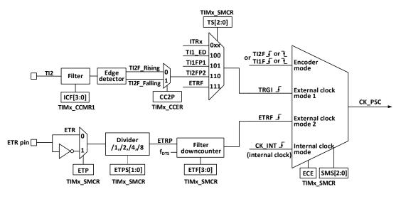
Figure 11-2 General-Purpose Timer CK\_PSC Source Block Diagram
