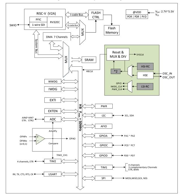
Figure 1-1 CH32V003 system block diagram
