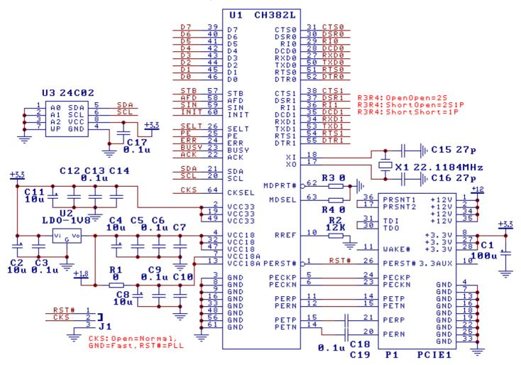
U3 is an optional external configuration chip, and the online configuration tool software for Windows system is available on the website.
