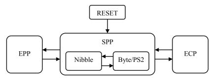
In the SPP mode, software can be used to control PCR and query PSR to realize transmission of Nibble, Byte and PS/2, etc. Refer to IEEE1284 specifications for the specific operation.
